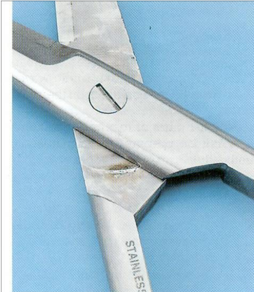
Fretting corrosion due to insufficient lubrication
